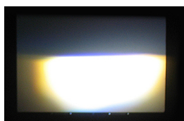
Beam shape with cut-off
